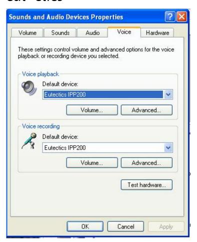
In the Voice tab choose the Eutectics Device (IPP200 in the above example) as the Playback and Recording - also click on the Volume Button and adjust the master volume to the highest level (you can make it lower later if desired).
